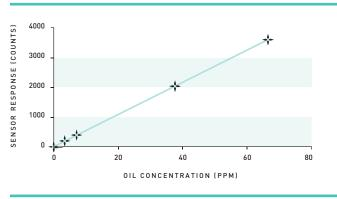
The sensor responds to various oils and generates positive correlations between the Fluorescence Index and oil densities. This means that the oil type can be detected from the density measurement.
