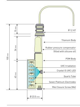
Schematic of the Idronaut conductivity sensor incorporating a Crystal IS LED for biofouling control.
