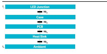
A simplified description of the thermal model for a Crystal IS LED package attached to a heat sink.
