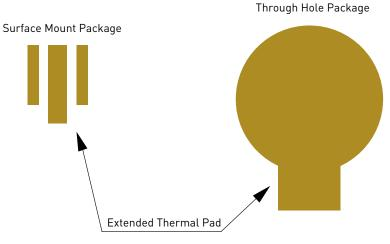
Suggested solder pattern showing extended thermal pad for measuring the solder point temperature.
