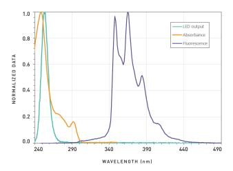
Absorbance and fluorescence spectrum of phenanthrene, with an overlay of the Crystal IS 255 nm Optan LED spectrum
