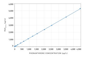
UviLux PAH+ sensor dose-response curve to phenanthrene, demonstrating the excellent linearity (R2 = 0.99998) that can be achieved across the full range from 0 - 4500  $\mu$ g/L, with integrated absorbance correction
