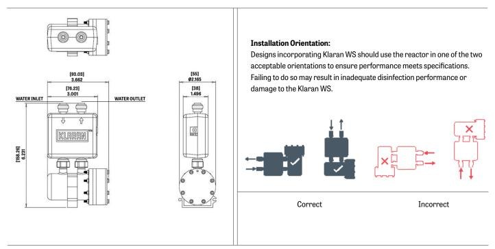
All dimensions are in millimeters. Unless noted otherwise, all dimensions have a tolerance of  $\pm$  0.05 mm.
